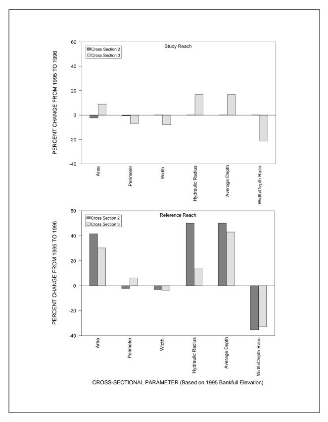
Figure 20. Summary of Changes in the Veety Farm Study and Reference Reach Channel Cross-Sectional Geometry Between 1995 and 1996
