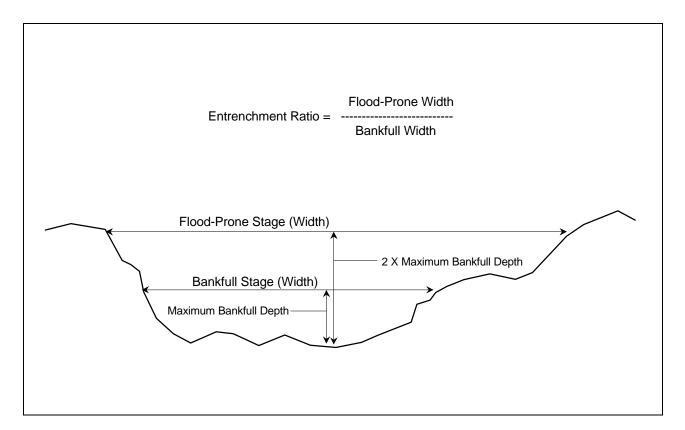
Figure 17. Illustration of Entrenchment Ratio Calculated From Bankfull and Flood-Prone Channel Width
