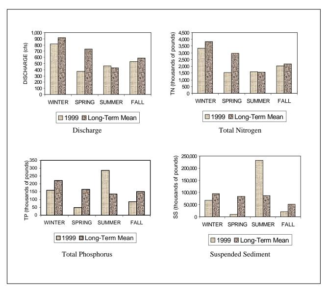
Figure 12. Seasonal Discharges and Loads of Total Nitrogen, Total Phosphorus, and Suspended Sediment at Conestoga, Pa., Calendar Year 1999
