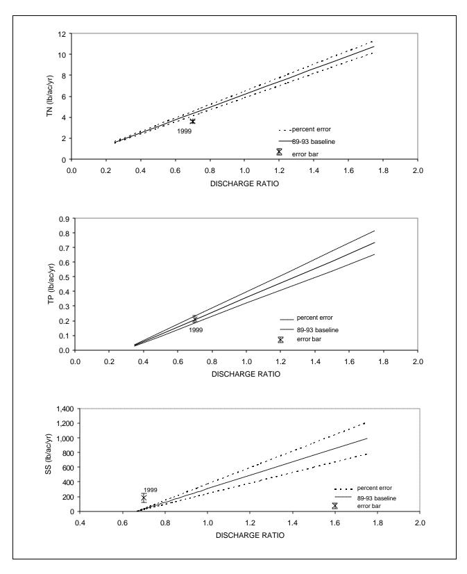
Figure 16. Total Nitrogen (TN), Total Phosphorus (TP), and Suspended-Sediment (SS)Yields, Susquehanna River at Towanda, Pa., 1989-93 and 1999
