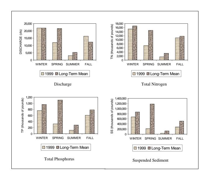
Figure 8. Seasonal Discharges and Loads of Total Nitrogen, Total Phosphorus, and Suspended Sediment at Danville, Pa., Calendar Year 1999
