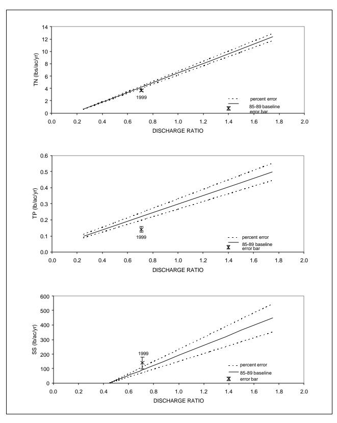
Figure 18. Total Nitrogen (TN), Total Phosphorus (TP), and Suspended-Sediment (SS) Yields, West Branch Susquehanna River at Lewisburg, Pa., 1985-89 and 1999
