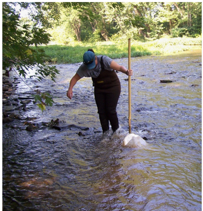
Commission staff using a D-frame kick net to sample bugs at Tuscarora Creek, Juniata Co., Pa., during low flow in September 2010.
