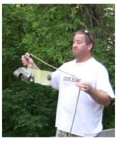
SRBC Environmental Scientist Kevin McGonigal displays USGS depth integrated sampler used to collect water that is analyzed for Total Nitrogen, Total Phosphorus, Total Organic Carbon, and Suspended Sediment.
