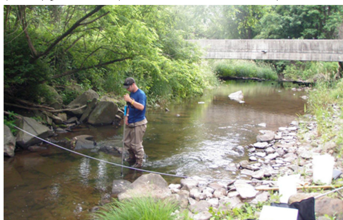
SRBC field staff measuring flow at Hills Creek at Crooked Creek, Pa. (HILL 0.2).
