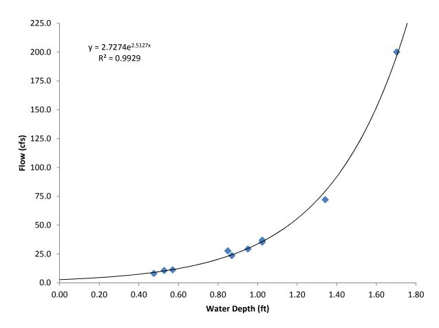
Figure 3. Preliminary Flow Rating Curve for the DRFT 2.0 (Driftwood Branch Sinnemahoning Creek) Flow Monitoring Network Station
