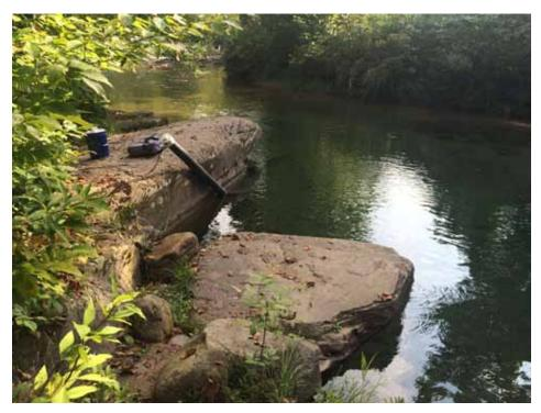
Data sonde at Pleasant Creek, Lycoming County, Pa. The data sonde is a multiparameter water quality sonde with optical dissolved oxygen and turbidity probes, a pH probe, and a conductance and temperature probe. The data sonde also includes a non-vented relative depth sensor. The entire unit is placed in protective housing and secured in free-flowing water at each site.
