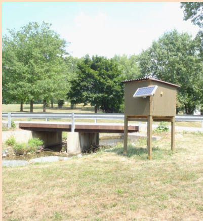
Continuous water quality monitoring and water auto-sampler station in the Cedar Run Watershed.
