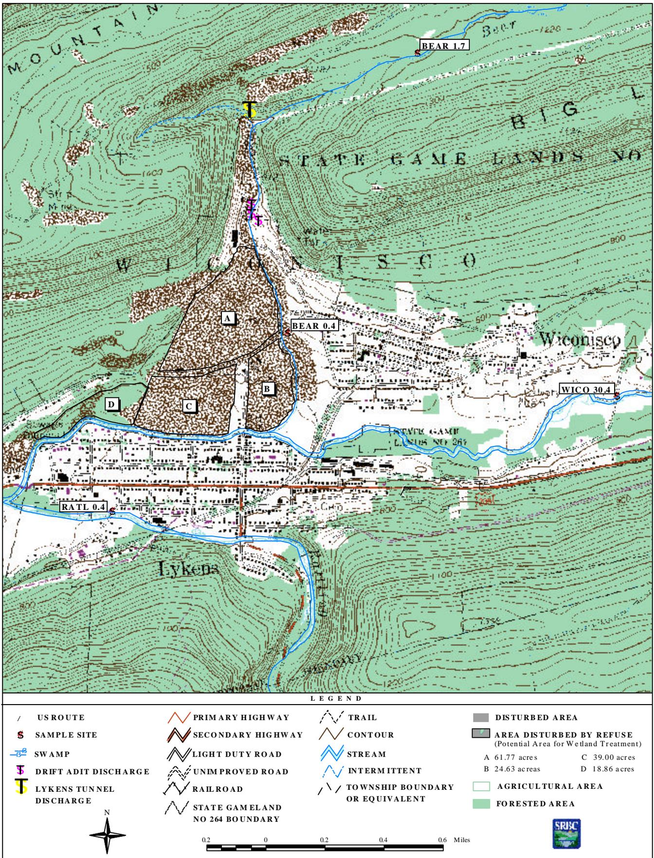
Figure 20. Mine Drainage Discharges and Potential Wetland Treatment Areas in the Bear Creek Watershed
