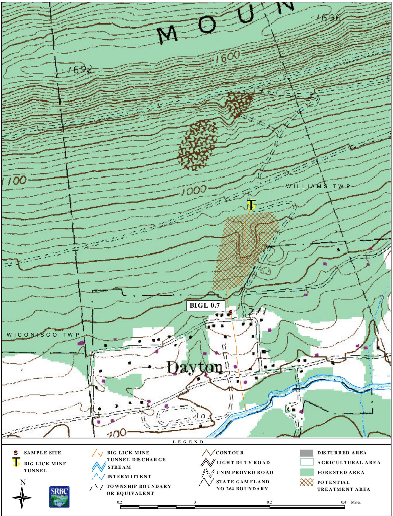
Figure 2. Big Lick Mine Tunnel Discharge and Potential Area for Settling Ponds and Wetland Treatment System
