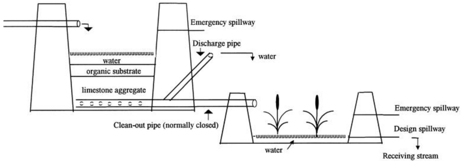
Figure 19. General Schematic of a Vertical Flow Pond Followed by a Constructed Wetland
