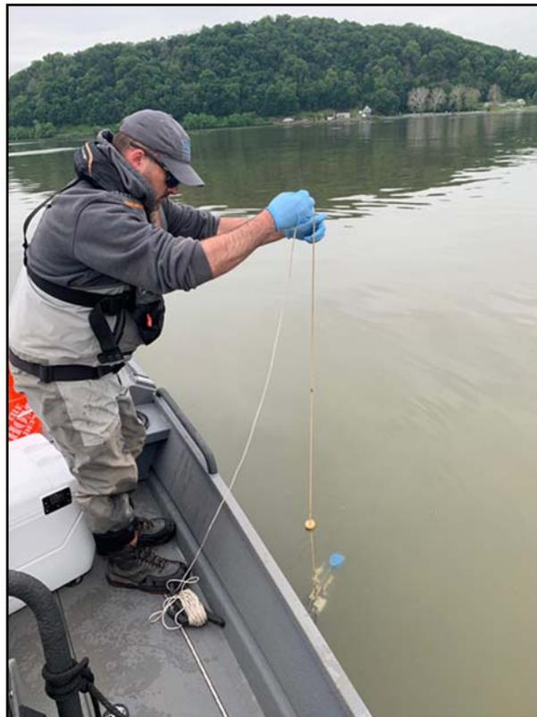
*Figure 3. SRBC Staff Using a Van Dorn Sampler to Collect a Depth-integrated Sample*
