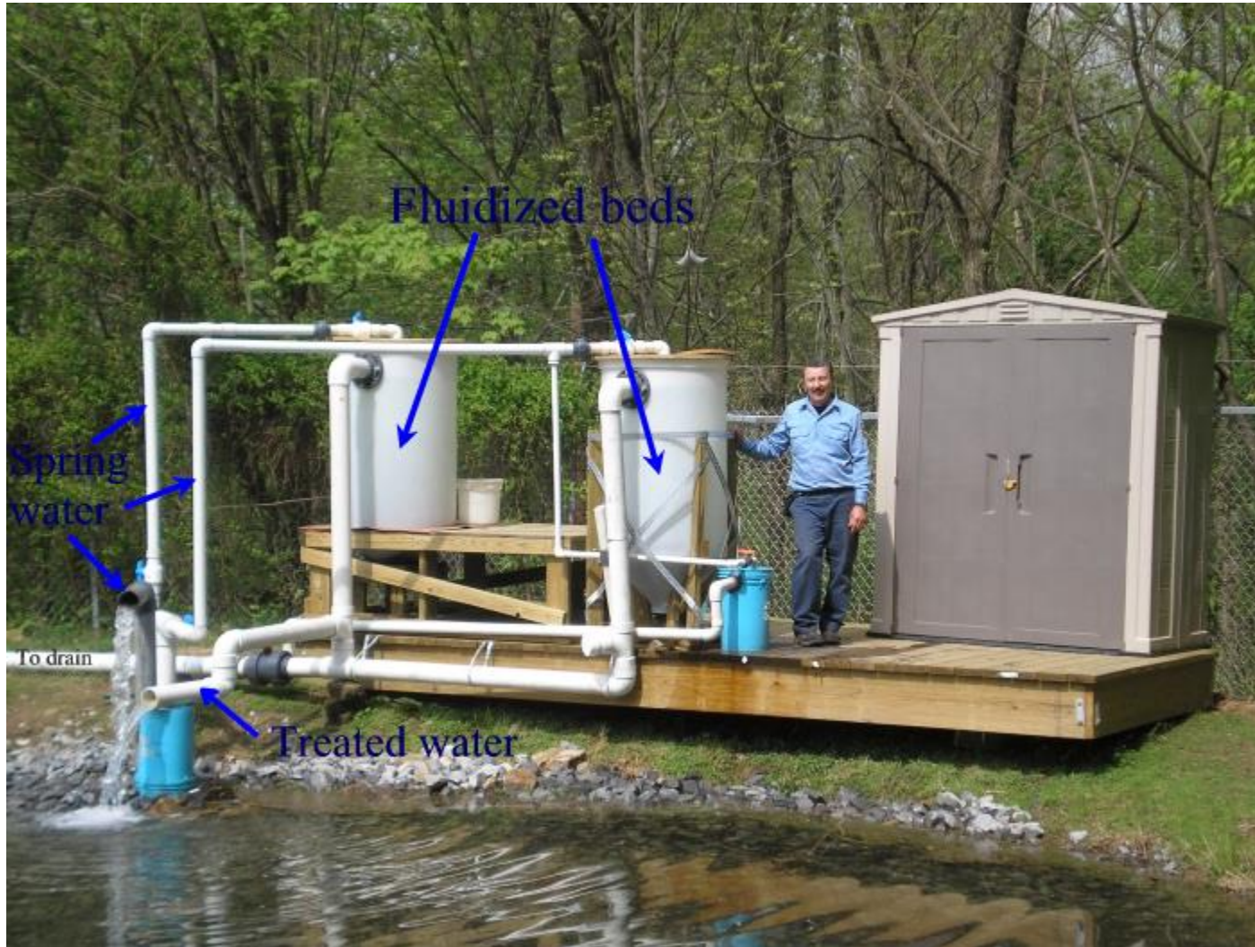
Figure 3. Photograph of the fluidized bed system installed at the Van Dyke Hatchery.
