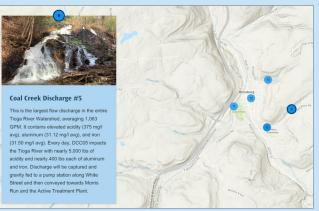
Visit the Tioga River AMD Treatment Plant Project story map for a tour of the study area and how the treatment plant will raise the pH of the drainage water to precipitate dissolved metals for capture and disposal.
