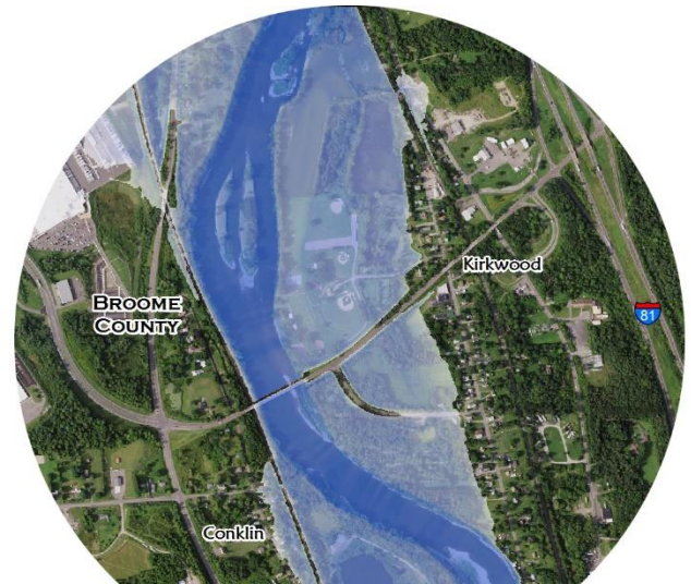
The map above shows the extent and depth of a flood resulting from stage 25.0' (record flood stage) at Kirkwood, NY.
