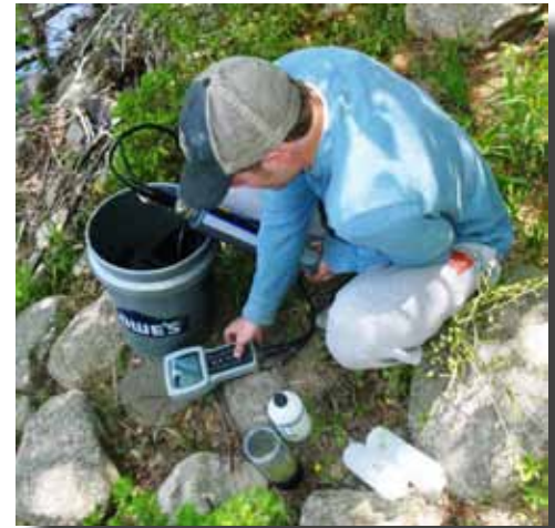
Matthew Shank, SRBC Aquatic Biologist, reads and records water quality data from a portable sonde.
