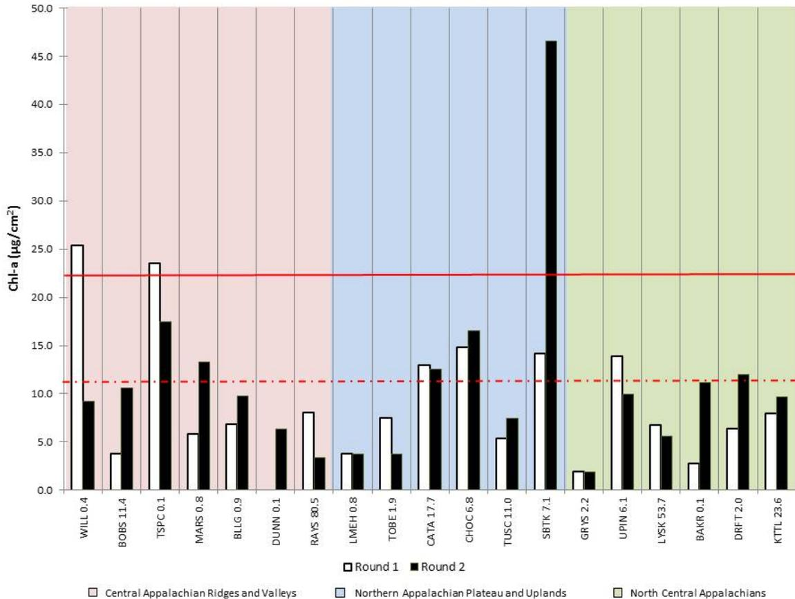
**Figure 14. Chlorophyll-a Concentrations at the Flow Monitoring Network Stations (Dashed Red Line Indicates Nuisance Level of Algal Growth; Solid Red Line Indicates Eutrophic Conditions)**
