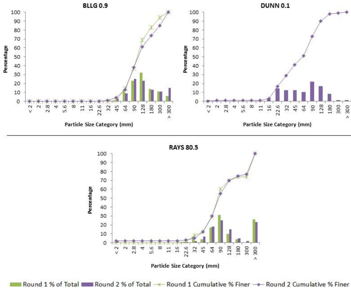
Figure 5. Substrate Particle Size Distribution (Percentage of Total and Cumulative Percentage Finer) for BLLG 0.9, DUNN 0.1, RAYS 80.5, Comparing Round 1 and Round 2 Pebble Count Data
