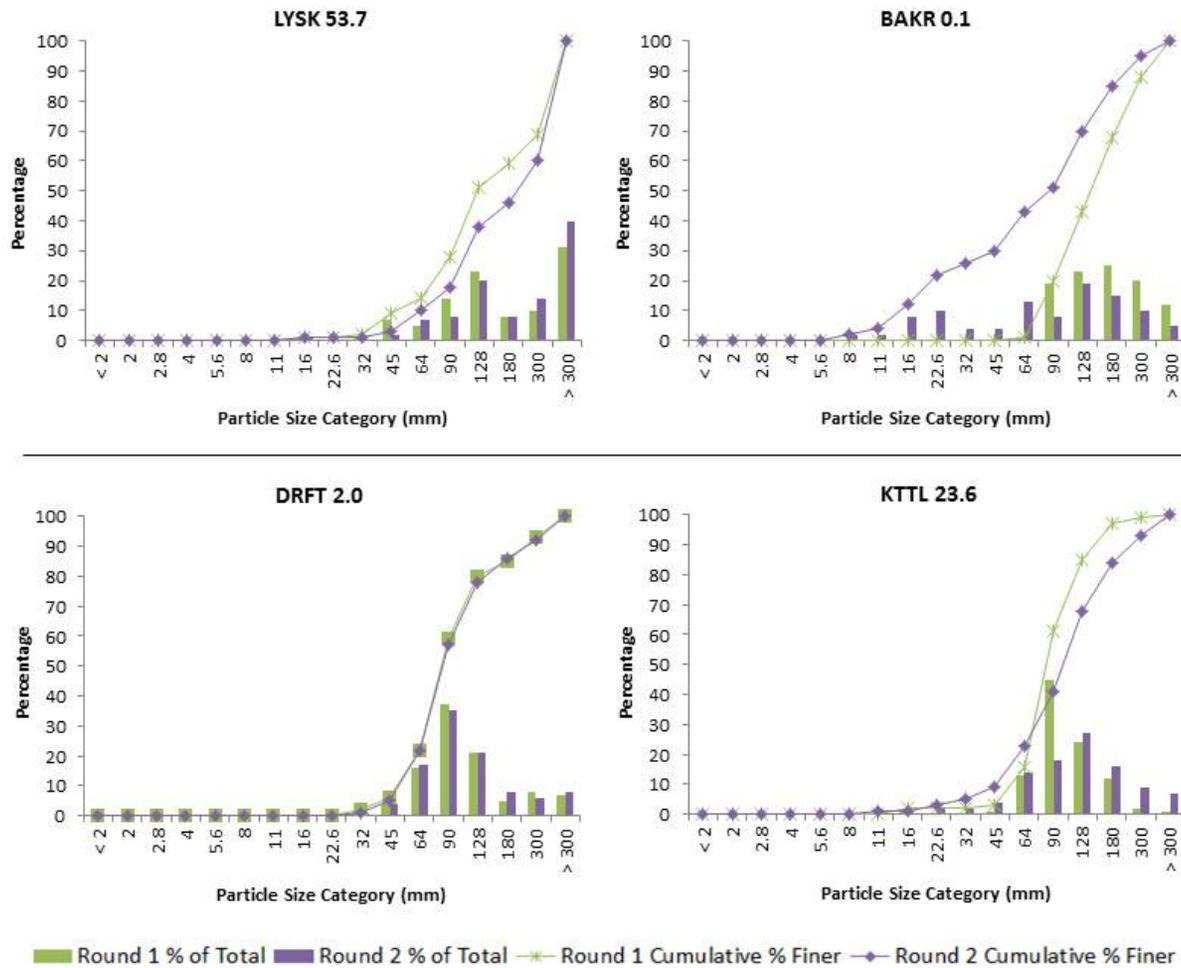
Figure 8. Substrate Particle Size Distribution (Percentage of Total and Cumulative Percentage Finer) for LYSK 53.7, BAKR 0.1, DRFT 2.0, and KTTL 23.6, Comparing Round 1 and Round 2 Pebble Count Data
