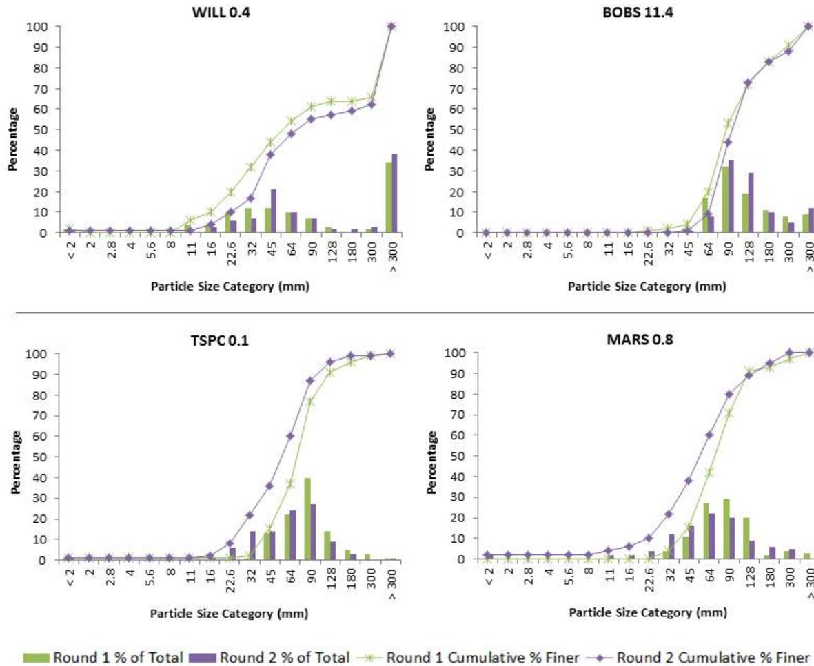
Figure 4. Substrate Particle Size Distribution (Percentage of Total and Cumulative Percentage Finer) for WILL 0.4, BOBS 11.4, TSPC 0.1, and MARS 0.8, Comparing Round 1 and Round 2 Pebble Count Data
