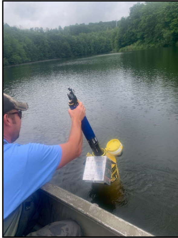
Figure 2. SRBC Staff Deploying Water Quality Monitoring Sonde Into the Buoy
