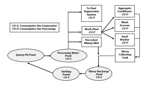
Water pumped into the processing water pond is also used at the tire wash before entering the scales and for dust suppression on the plant roadways as needed.
